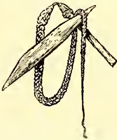
A DRIVER'S WHIP, AND SPRAG FOR SCOTCHING THE WHEELS OF THE CAR.
